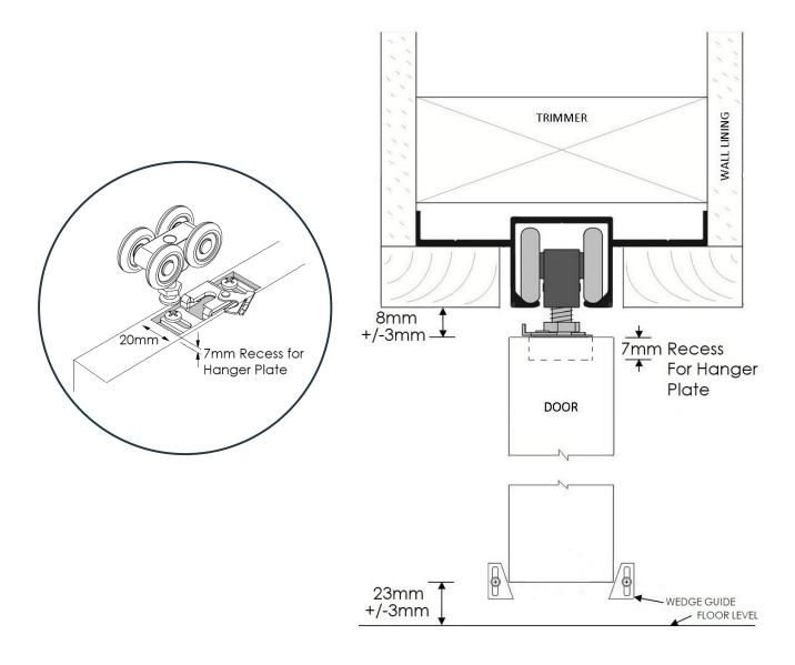
With the new hanger plate design which is recessed into the top of the door by max. 7mm, you can now achieve that sophisticated and architectural look with clearances of a minimum of 5mm (depending on the clearances required under the door) between the track and the top of the door, eliminating the need for timber pelmets.
