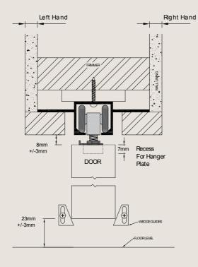
PRO-LINE 60 - LESS THAN FULL HEIGHT (UNDER BULKHEAD)
