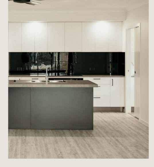
Using a sliding door to the pantry in this application reduces any obstruction caused by your typical swing door that would swing either into the pantry or kitchen space.
