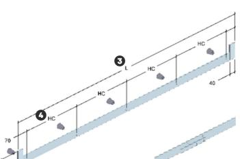
6S Spacer supplied for each hole in track with 10 x 100mm hex head coach screw
