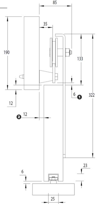
Splice/Join is supplied with 2 fixing bolts for tracks over:
