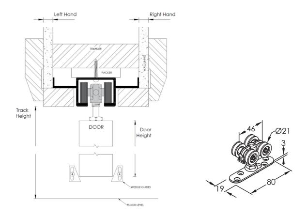
The Concept<sup>™</sup> unit allows for a minimal 10-15mm gap between the track and the top of the door. Perfectly suited to full height openings, it is also available for standard height doors as single or double door units.
