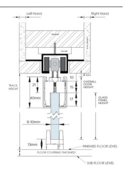
FRAMELESS GLASS CAVITY SLIDER LESS THAN FULL HEIGHT (WALL ABOVE)
