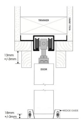
The Hercules<sup>™</sup> cavity system is suitable for single doors sliding to one side or double doors sliding either side on a single track.
