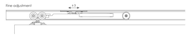
6 Adjust catch plate as required. Secure in final position with the 3rd screw.
