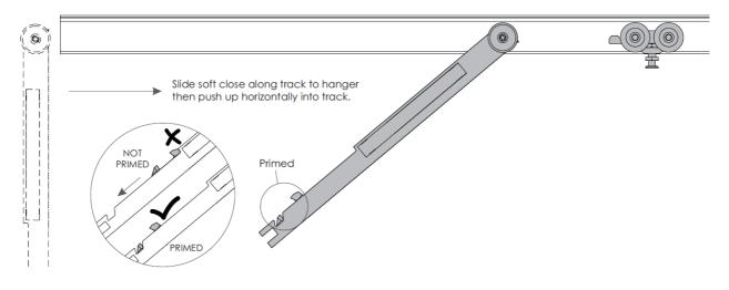
2 Insert 2nd hanger & attached hanger to soft close with cap screw. Install panel as per sliding door system instructions.
